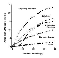
**Figure 4**. Biodegradability of biodegradable plastics in controlled soil at 35<sub>1</sub>C.
